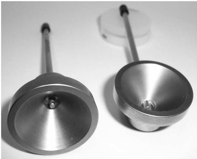
Fig. 2. Photograph of the vertical (left) and horizontal (right) 3 cm in diameter Leipzig applicators (H3 and V3).
